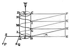
BH, GK, IF. If now the rectangle EC be wrapped upon the cylinder so that BE coincides with the circumference of the base, the points E, H, K, F, will respectively fall upon the points B, G, I, C, of the cylinder, and the lines BH, GK, IF, will trace out on its surface the continuous spiral thread BLGMINC winding round the cylinder, and everywhere inclined at the same angle to its base. If we now suppose this thread to become protuberant, we shall have the screw traced on the cylinder.
